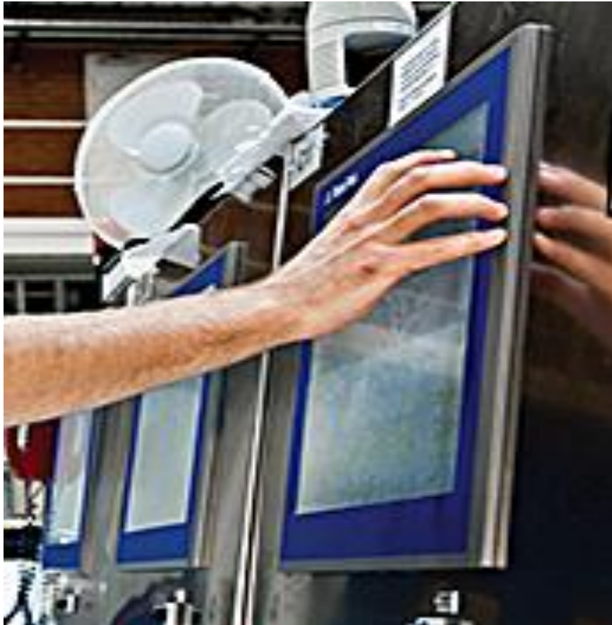
Figura 11 - Painel HMI Fonte – SCHUG (2016)
