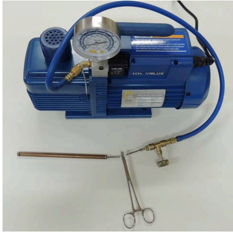
Figure 5. Vacuum pump and the thermosyphon.
