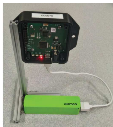
Figure 3.18: Pozyx anchor using a power bank as energy source.
