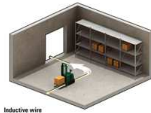
Figure 2.11: Localization and navigation system based on wire guidance [25].
