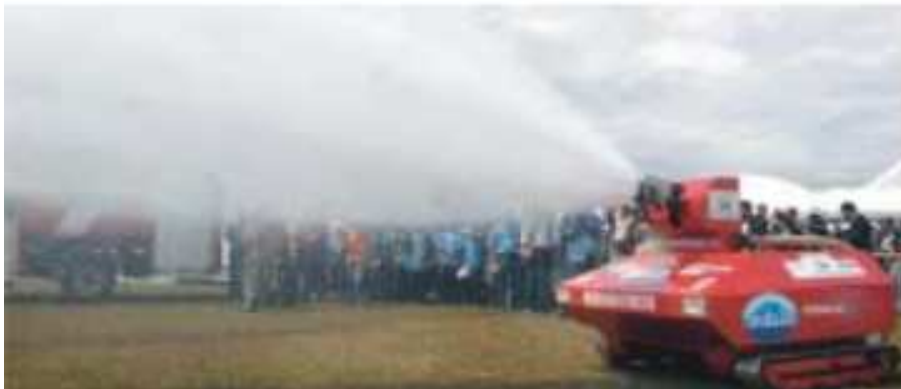
Figure 2.3: SACI robot emitting a jet of water to combat the fire [11].
