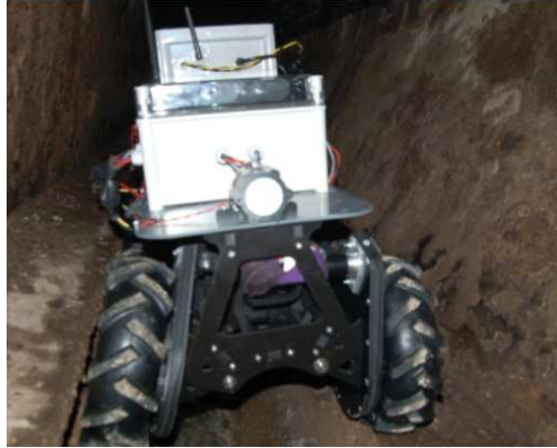
Figure 2.2: SIAR robot conducting an inspection in a sewer[10].
