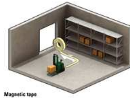
Figure 2.12: Localization and navigation system based on strip guidance [25].
