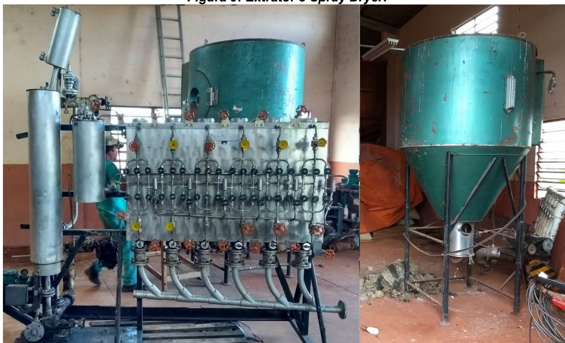
Figura 9: Extrator e Spray Dryer .
