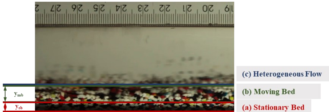
Figure 18 – Detail of the flow with a stationary bed, indicating the (a) stationary bed layer, (b) moving bed layer and (c) heterogeneous flow for Re = 20,000 employing water as the working fluid.
