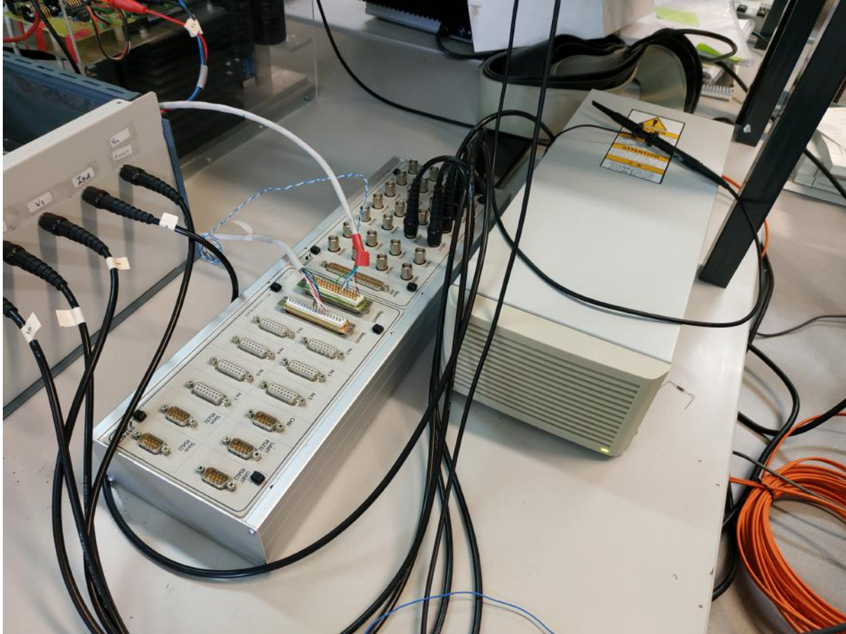
Figure 4.5: DS1103 Controller Board box and connections'panel
