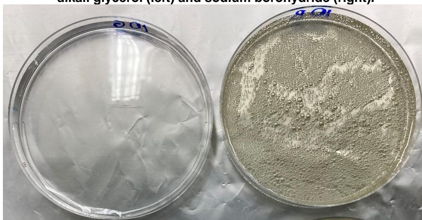
Figure 21: Evidence of reaction observed by the change in colour of the reducing solutions of alkali glycerol (left) and sodium borohydride (right).
