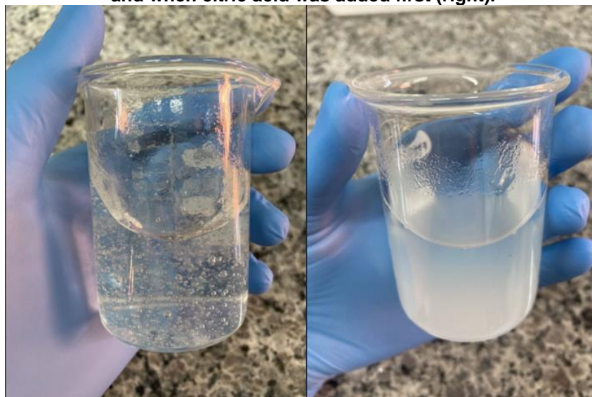
Figure 16: Differences in the aspect of the solutions when the cellulose was added first (left) and when citric acid was added first (right).
