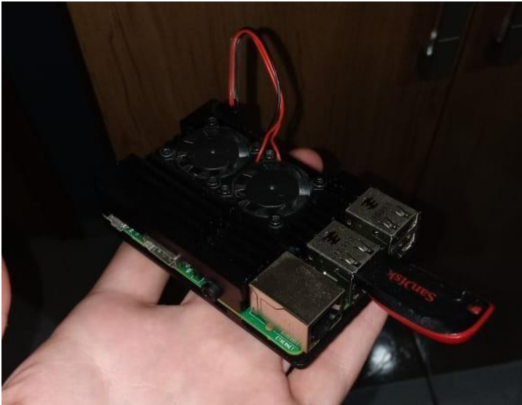
Figura 112 – Raspberry pi com cooler e retropie
