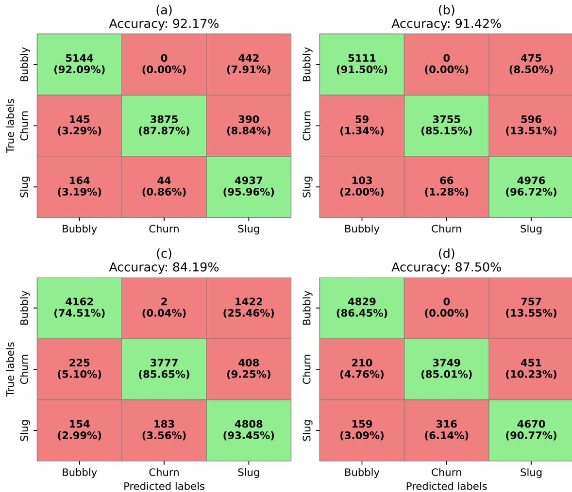
Figure 35 – Confusion matrices for models trained with the HZDR dataset and tested with the TUD dataset. (a) ResNet. (b) LSTM-FCN. (c) TSTPlus. (d) *MoG-SVM*
