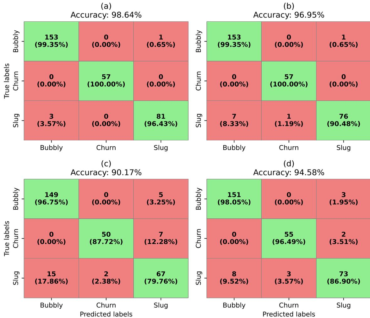
**Figure 21 – Confusion matrices for models trained with the HZDR dataset. (a) ResNet. (b) LSTM-FCN. (c) TSTPlus. (d) *MoG-SVM*.**
