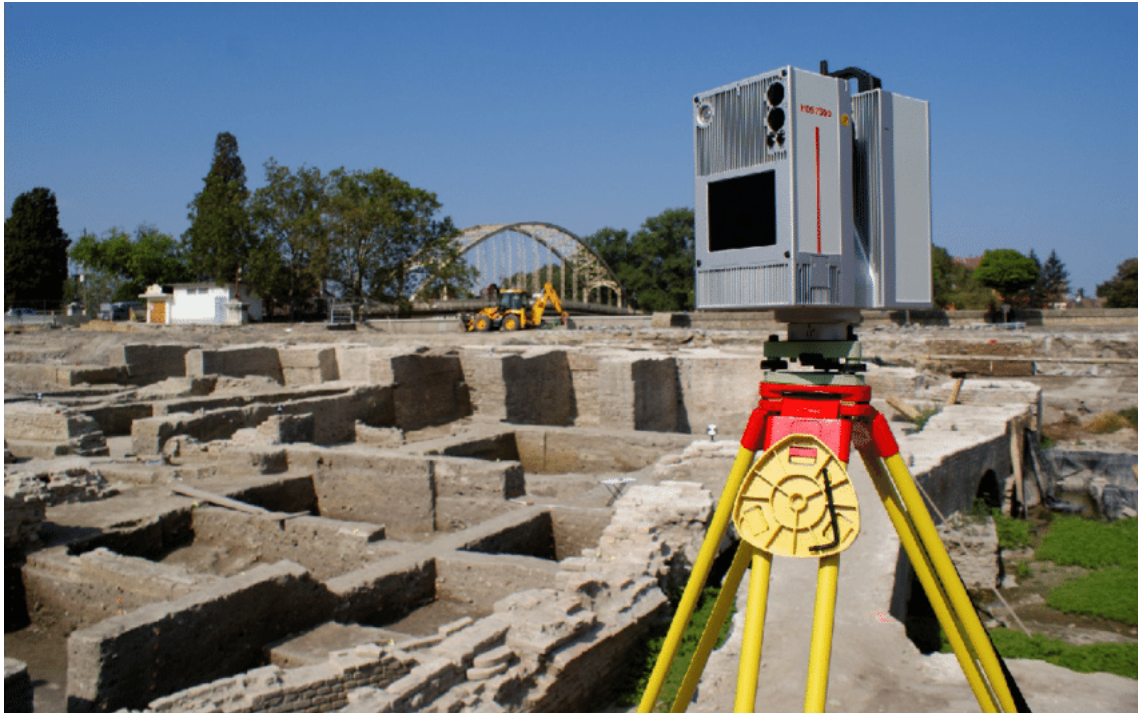
Figure 10 – Terrestrial laser scanner in operation at the field survey at Dunakapu Square, Győr.
