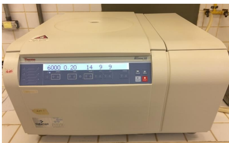
Figura 23 – Centrífuga Thermo Scientific ® (modelo Heraeus Megafuge 16R ).
