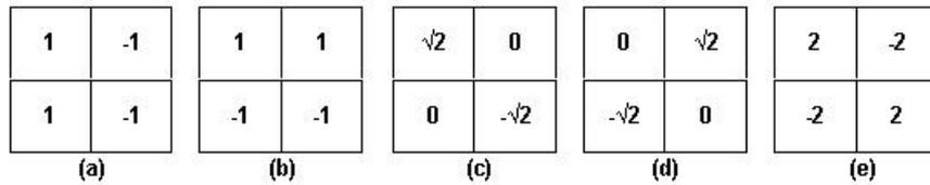
**Figure 3: Five filters for edge detection (a) vertical (b) horizontal (c) 45-degree diagonal (d) 135-degree diagonal (e) non-directional edge**
