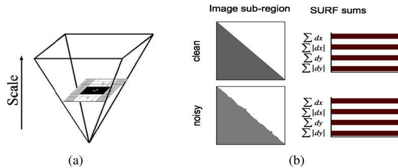
**Figure 1: (a) Analyzing the scale space by up-scaling the filter size using a pyramid scheme (b) Image sub-region and its sum of intensity patterns**
