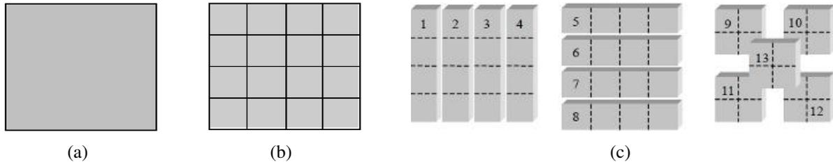
**Figure 4: Face image partitions scheme for feature extraction (a) global image (b) Sub-images for local edge histograms (c) Subsets of sub-images for semi-global edge histograms**
