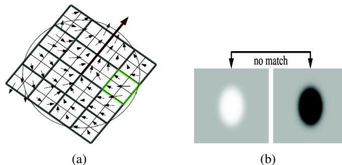
**Figure 2: (a) Descriptor construction using oriented quadratic grid with 4 x 4 square sub-region and Haar wavelet responses ( $\sum dx, \sum dy, \sum | dx |, \sum | dy |$ ) around an interest point (b) Interest point matching using contrast type**
