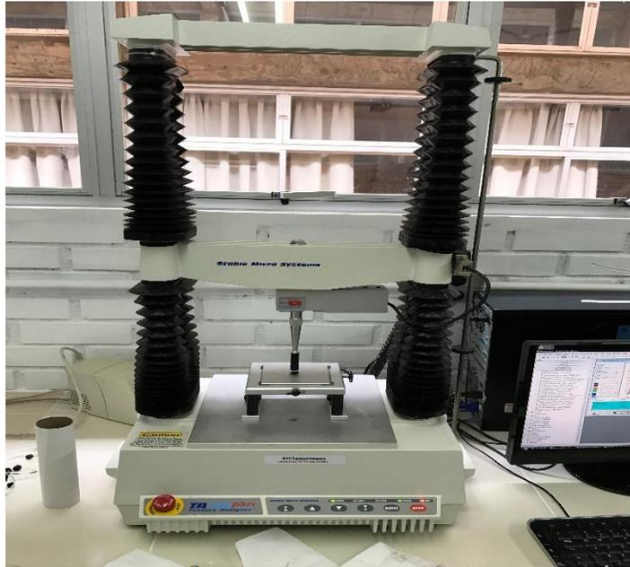
**Figura 7.** Texturômetro TA-HD PLUS.
