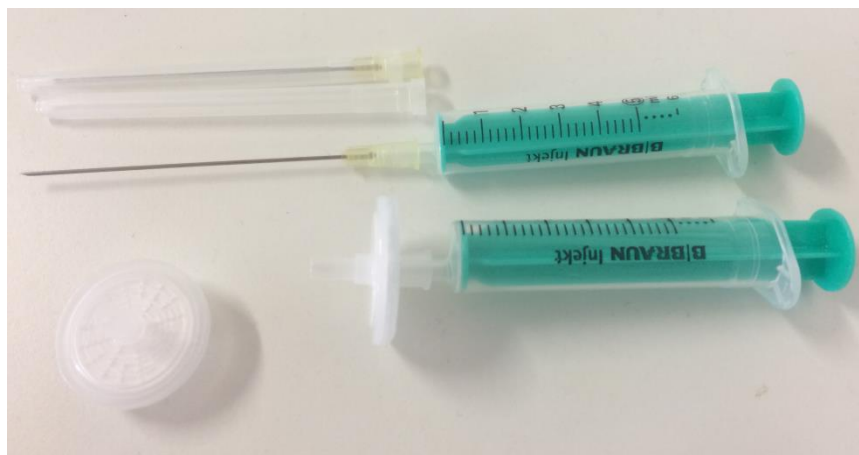
Figure 3.2: Syringes and filters used to collect the samples from the solutions.
