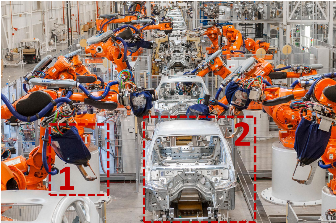
Figure 1 – Example of a multi-operated robotic welding assembly line: robots holding spot welding tools (1) and a vehicle's body (2) are illustrated.
