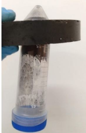
Figure 9 - Demonstration of the magnetic properties. All material, including the Falcon tube, is supported by a magnet.
