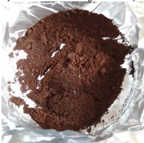
Figure 8 - Catalyst recovered for storage after completing step 3 (H).
