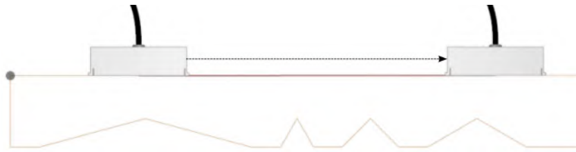
Figure 26 – Schematic of the acrylic specimen inspected and the probe’s trajectory. The trajectory starts in x = 45 mm and goes to x = 170 mm in steps of 5 mm. At each position an FMC acquisition is done.
