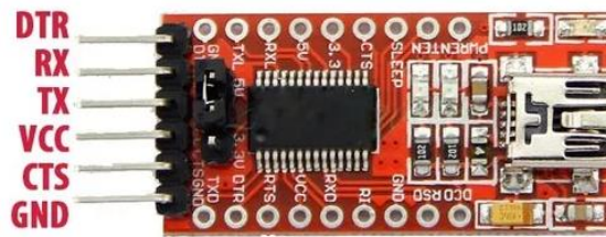
Figura 17 – Placa FTDI FT232RL conversor USB serial
