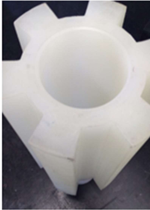
Figure 7. Drill bit model manufactured in Polypropylene with grooves. External diameter of 130 mm.
