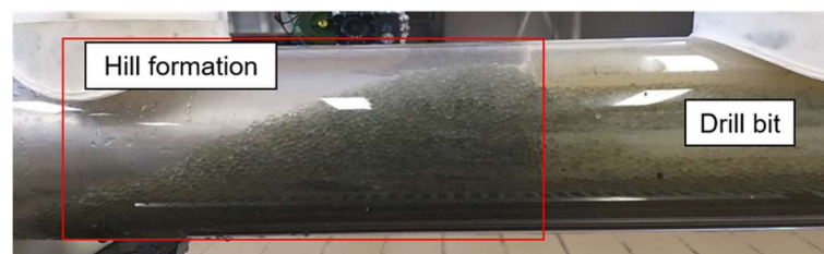
Figure 18. Cuttings hill formed after displacing the column to the left with a 33 mm (23.6%) cuttings bed height at 10 cm/s displacement speed without rotation. The hill reached 20 cm long.
