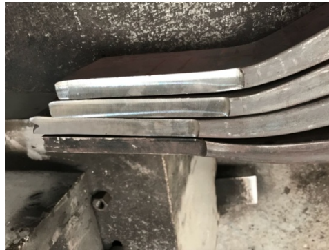
Figure 13 – Springs after face milling. Source: Author.
