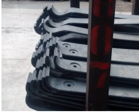
Figure 8 – Springs after semi-fold. Source: Author.
