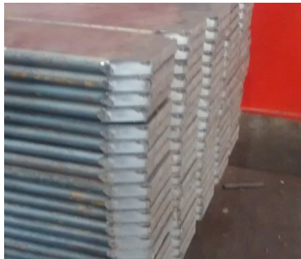
Figure 11 – Springs after tip removal. Source: Author.
