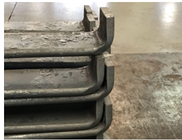
Figure 9 – Springs after fold. Source: Author.
