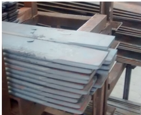
Figure 4 – Springs after conventional lamination. Source: Author.
