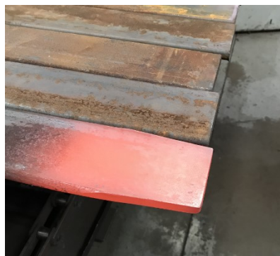
Figure 7 – Springs after chamfering. Source: Author.
