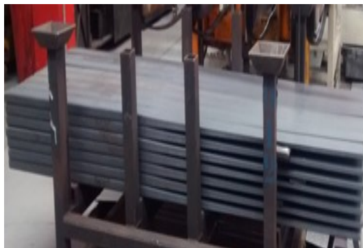
Figure 3 – Springs after parabolic lamination. Source: Author.
