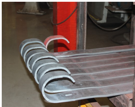
Figure 6 – Springs after second fold. Source: Author.
