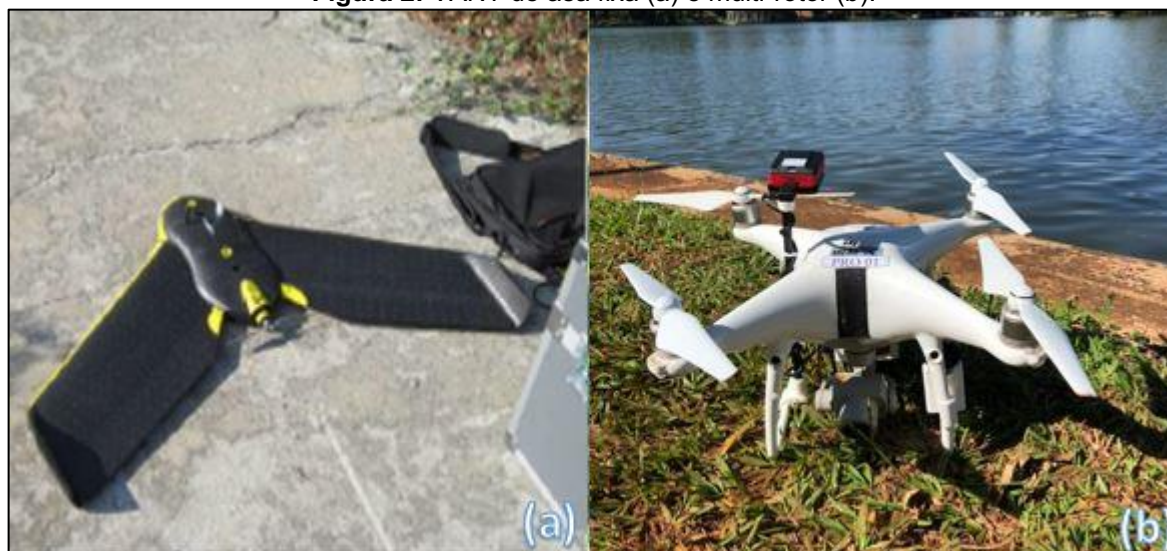
Figura 2: VANT de asa fixa (a) e multi-rotor (b).
