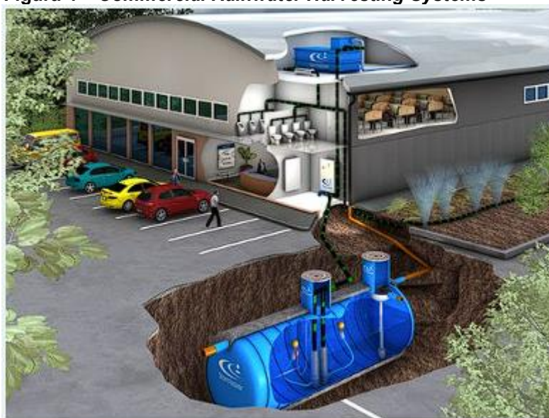
Figura 4 – Commercial Rainwater Harvesting Systems
