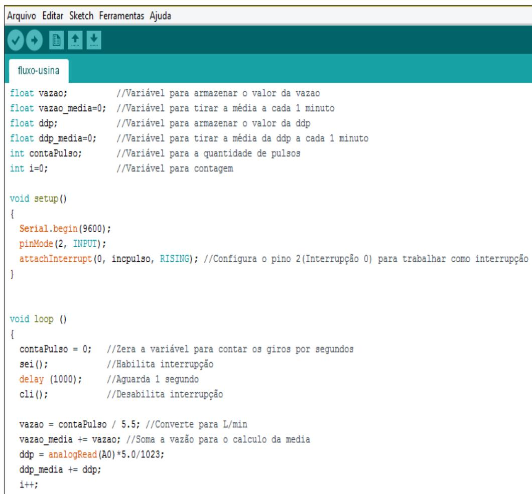
The image shows a screenshot of the Arduino IDE interface. At the top, there is a menu bar with 'Arquivo', 'Editar', 'Sketch', 'Ferramentas', and 'Ajuda'. Below the menu bar is a toolbar with icons for saving, running, uploading, and downloading. The main area displays a sketch named 'fluxo-usina' with the following code:
