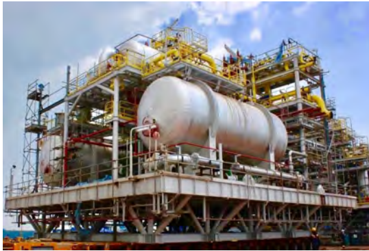
(a) Actual three-phase separator. Source: Adapted from (5)
