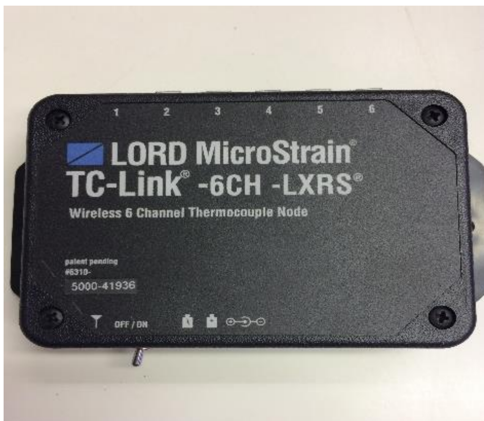
Figura 6: Sensor wireless LORD MicroStrain.
