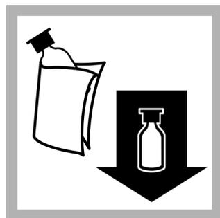
6. When the timer expires, wipe the blank and insert it into the cell holder.
