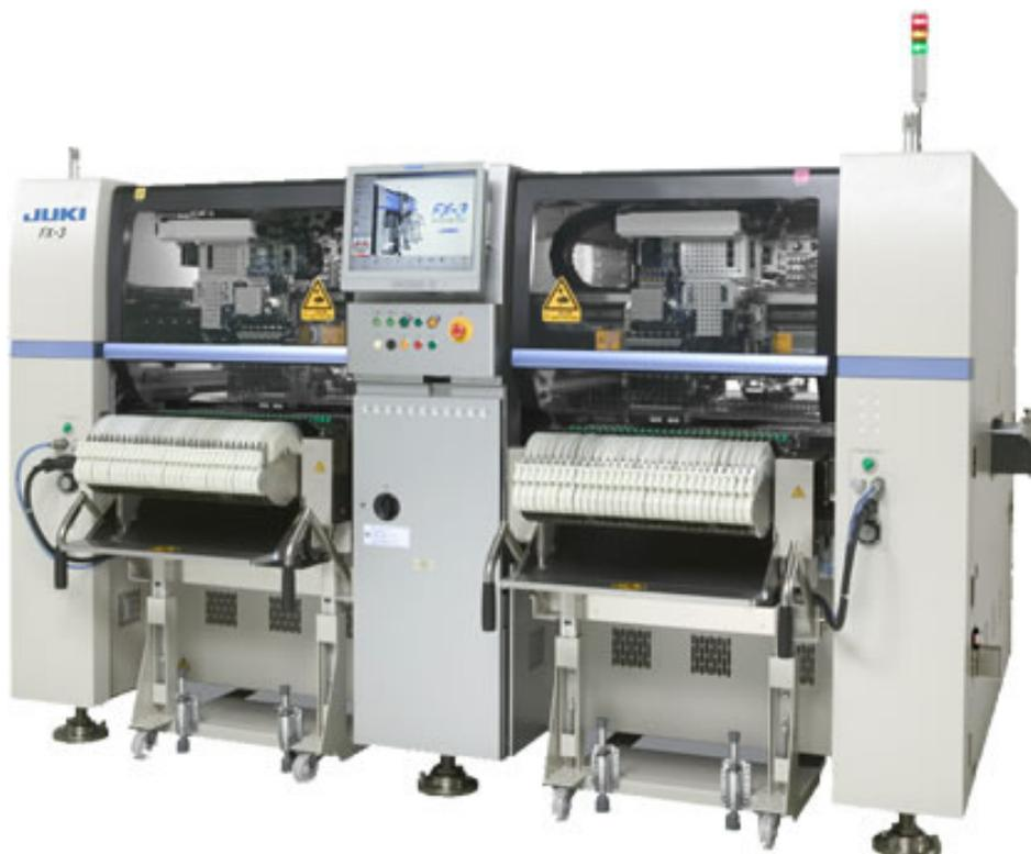
**Figura 20 - Máquina *Pick and Place***
