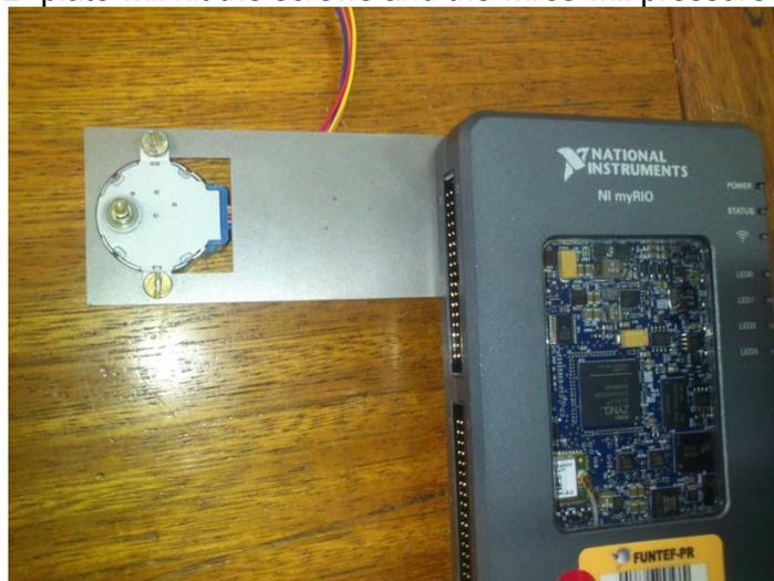
4. Do the same on the "L" plate. Fit the L plate on the first stepper and the sensor tower on the second stepper.
